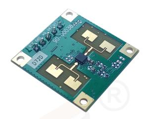
24GHz millimeter wave radar sensor PIR motion monitoring module LD116 small size, low power consumption, wide detection
